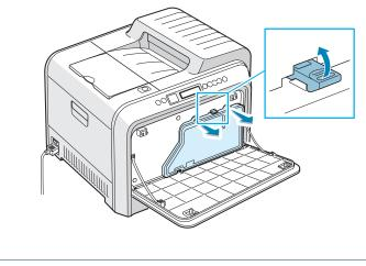
**NOTE**: Make sure that you lay the waste toner container on a flat surface so that the toner does not spill.
